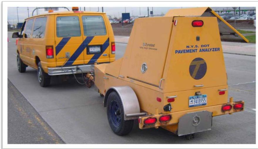
Figura 3-18 - Falling Weight Deflectometer (FWD)
